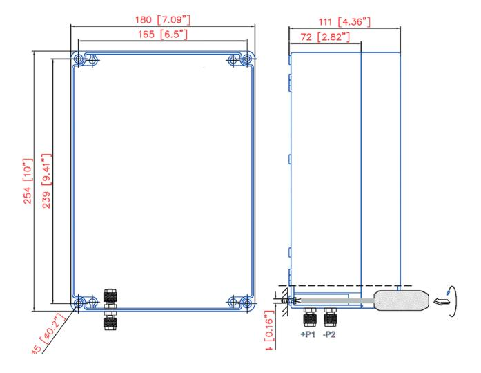
Material: PS thermoplastic/RAL 7035 Temperature: -10°C÷70°C
